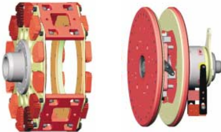
Figure 2: Drive showing magnet rotor assembly removed from conductor assembly.
