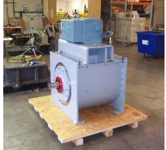
MagnaDrive Totally Enclosed ASD for the DOE Hanford Site.
